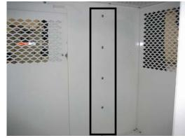
Location on inside of K9 assembly where rear partition will bolt to using 1/4" x 3/4" carriage bolts and nuts
